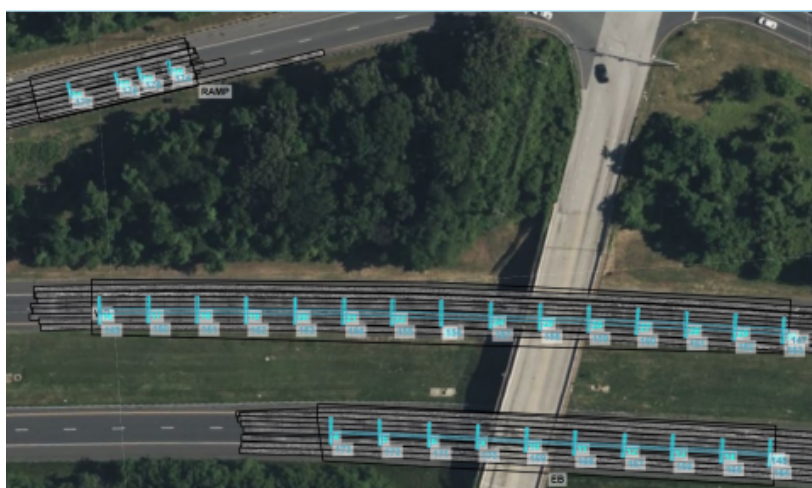
Joint and dowel-bar locations
